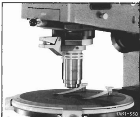
Fig. 22 ORTHOPLAN-POL with objective centring clutch
